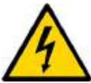
Warning; Electricity Code W012
